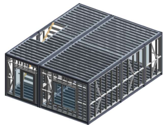
Steel View Ground Floor
