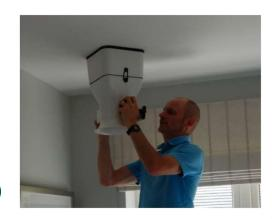
They shall then proceed to take measurements to establish that the commissioned system complies with the satisfactory presented design, i.e. achieves the design flow rates (I.S. EN 14134:2019 Ventilation for buildings – Performance testing and installation checks of residential ventilation systems).
