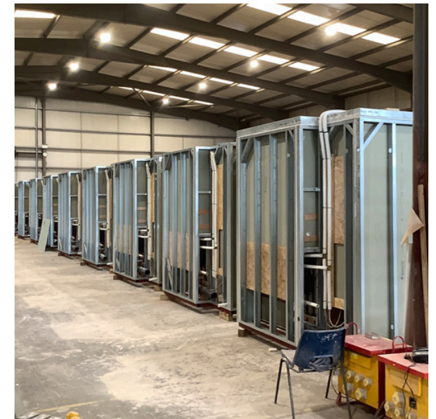
Bathroom Pods being manufactured for the scheme
