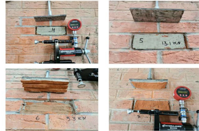
Determination of Bond Strength by Pull of Test
